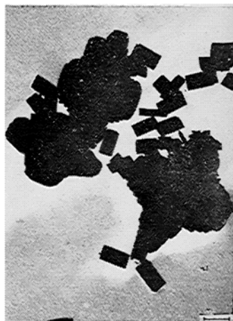
Photo. 15. Produced crystals (Cr-shadowing, \times 5,000 )
