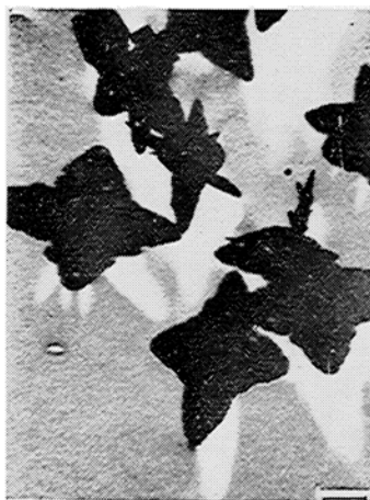
Photo. 14. Crystalline nuclei (Cr-shadowing, \times 5,000 )
